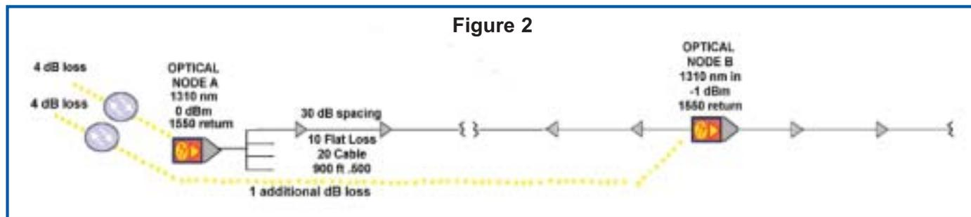
node. We are also going to assume that in the RF portion of the plant the amplifiers are spaced at 30 dB with 10 dB of flat loss and 20 dB of .500 or 900 feet between amplifiers.
