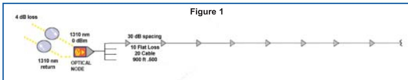
0 dBm with a fiber loss of 4 dB or a little over 6 miles and a 1310 return as shown in Figure 1.
