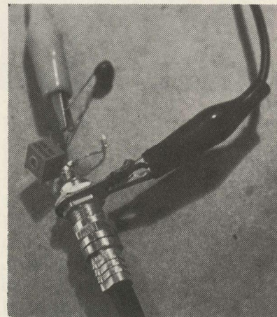
THE FIVE PART MODULATOR "thrown together" to get video into the Gunnplexer transmitter.
