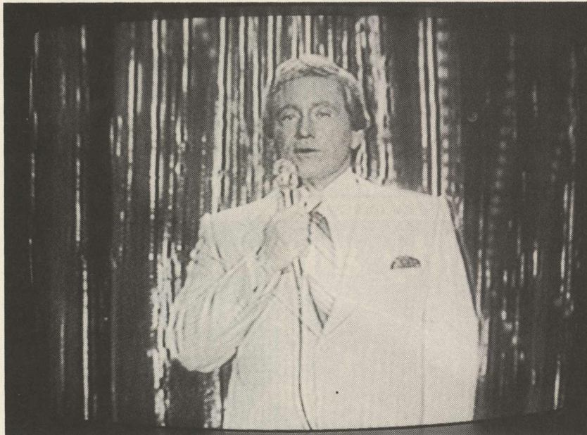
MERV VIA 10.38 GHz experimental Gunnplexer microwave; video and audio taken from a CATV demodulator, fed through the Gunnplexer system, and then demodulated and fed back into CATV channel 2 modulator and displayed on a normal home receiver. Could you sell it?
